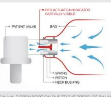
VALVE IN HALF OPEN POSITION DUE TO THE PRESSURE BALANCE BETWEEN BAG AND PATIENT'S AIRWAY
