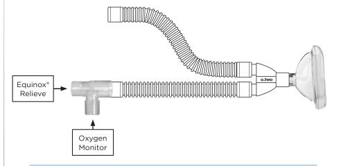
Fig. 2 - Connecting the Oxygen Monitor
