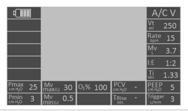
Figure 07 - A/C V mode screen w/ default parameters (Child setting)
