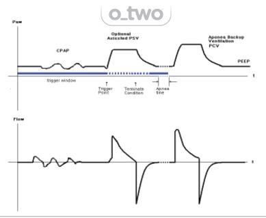
Figure 13 - CPAP ventilation waveform
