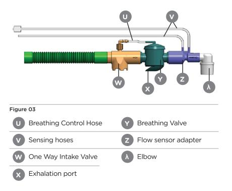
**Note:** To avoid entanglement of the patient circuit tubing and pressure sensing hoses during movement of the patient, the pressure sensing hoses and the 22mm corrugated hose are contained within in a close fitting, non-woven fabric sheath.
