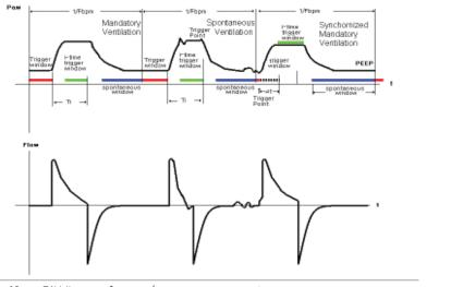
Figure 12.a - BiLVL waveform w/o pressure support
