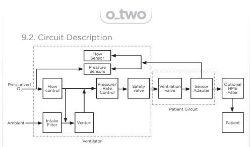
When a gas source (medical oxygen) is supplied to the e700<sup>®</sup> ventilator via the gas input connection, the gas will flow into the Flow control valve which is used to control both the flow and rate of ventilation.
