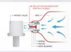
VALVE IN HALF OPEN POSITION DUE TO THE PRESSURE BALANCE.
