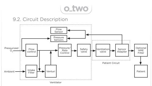
When a gas source (medical oxygen) is supplied to the e500 ventilator via the gas input connection, the gas will flow into the Flow control valve which is used to control both the flow and rate of ventilation.
