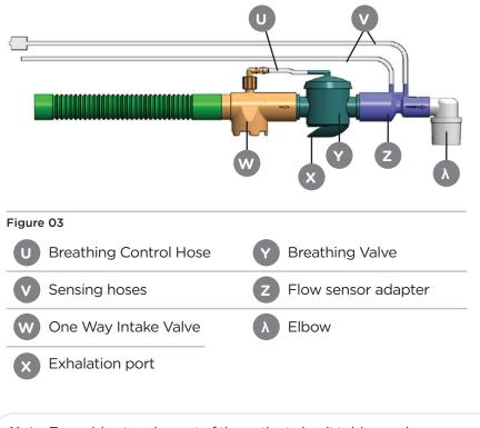
**Note:** To avoid entanglement of the patient circuit tubing and pressure sensing hoses during movement of the patient, the pressure sensing hoses and the 22mm corrugated hose are contained within in a close fitting, non-woven fabric sheath.
