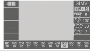
Figure 09 - Showing selected parameter with solid contrasting background
