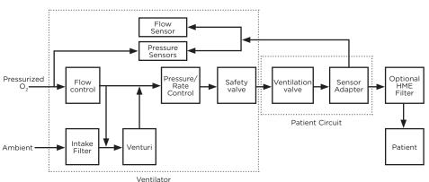
When a gas source (medical oxygen) is supplied to the e500 ventilator via the gas input connection, the gas will flow into the Flow control valve which is used to control both the flow and rate of ventilation.
