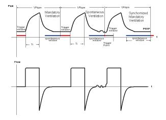
Figure 10 - SIMV waveform
