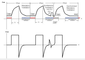
Figure 11.b - SIMV waveform with pressure support
