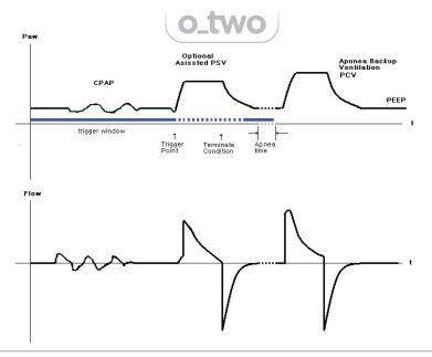
Figure 13 - CPAP ventilation waveform
