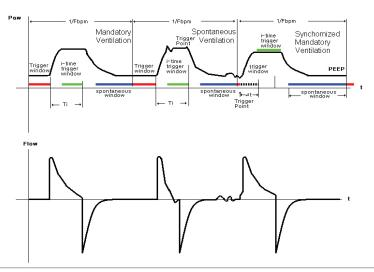
Figure 12.a - BiLVL waveform w/o pressure support
