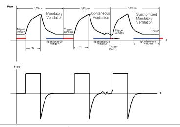
Figure 11.a - SIMV waveform w/o pressure support
