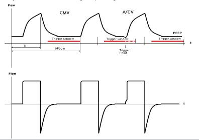
Figure 10.a - A/C V waveform with volume control
