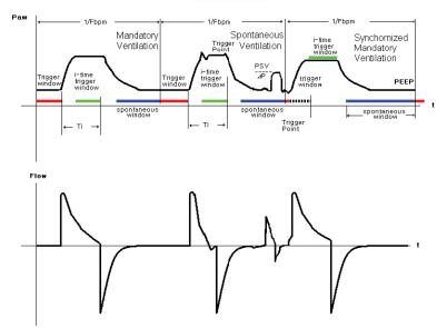
Figure 12.b - BiLVL waveform with pressure support
