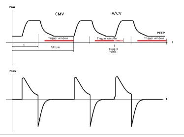
Figure 10.b - A/C V waveform with pressure control
