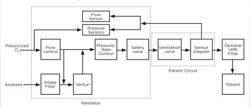
When a gas source (medical oxygen) is supplied to the e700° ventilator via the gas input connection, the gas will flow into the Flow control valve which is used to control both the flow and rate of ventilation.
