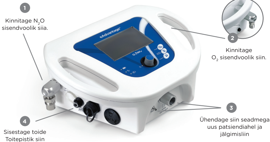
Joonis 1. Connecting the Supply hoses, Patient Circuit and Power Supply
