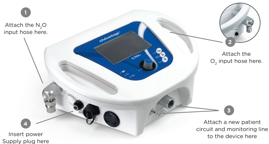
Fig. 1 Connecting the Supply hoses, Patient Circuit, and Power Supply
